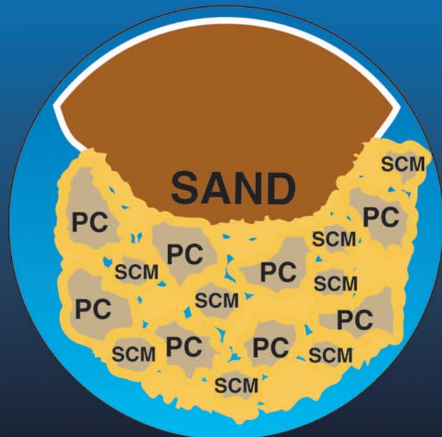
*When supplementary cementitious materials (SCMs) are added, particles pack more tightly within the voids and additional glue forms from the hydration process. With fewer voids, the concrete is less permeable and stronger.*
