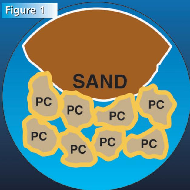
*When ordinary portland cement hydrates, calcium silicate hydrate (CSH) is formed (shown in yellow), and serves as the glue holding concrete together. However, gaps provide pathways for moisture to penetrate and reduce strength.*
