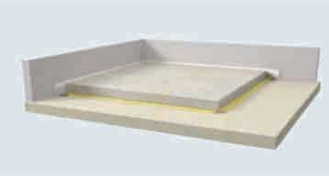
Floating or Unbonded system
